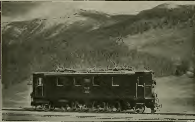
ELECTRIC LOCOMOTIVE OF 600 H. P. USED ON THE ELECTRIC LINE LEADING FROM BEVERS TO SCHULS-TARASP
